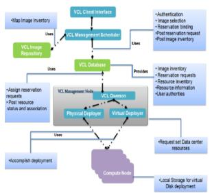
Figure 1: VCL Architecture overview plus Workflow description
